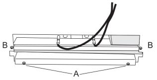
Remove the 2 screws 'A' and allow the plate to drop down. Remove the 2 screws B, lower the upper plate and remove through the slot in the cooker back.
